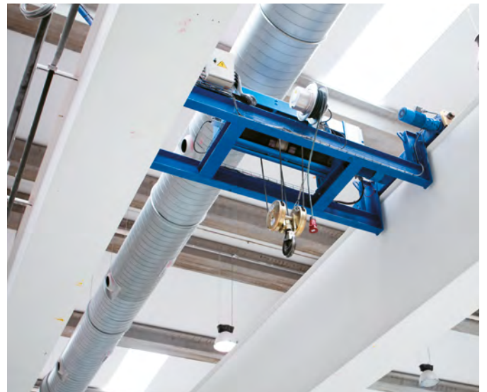
TROLLEY "CRADLED" BETWEEN TWO GIRDERS allowing lower total headroom for the crane.
