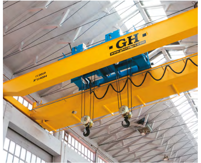
CRANE WITH TWO HOISTS ON ONE TROLLEY with the two hoists having the same capacity or different capacities.
