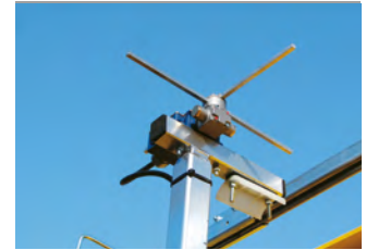
TROLLEY AND CRANE TRAVEL LIMIT SWITCHES
