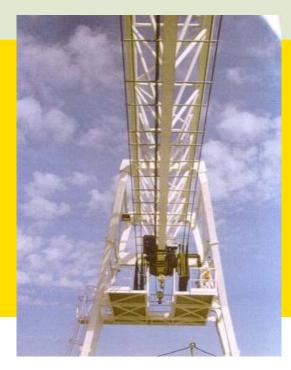
Portal Cranes with a lattice structure, are designed to reduce the maximum surface area against wind resistance, optimising its power for the long travel movement.
